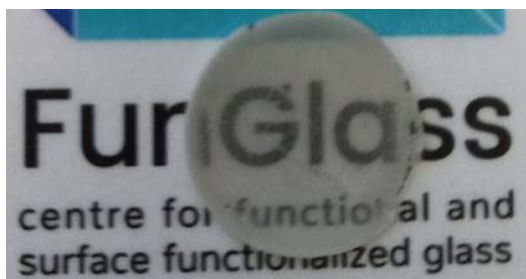
Fig. 1 Bulk glass in the composition of YAG + 24 wt. % Al 2 O 3 sample sintered in viscous flow.
