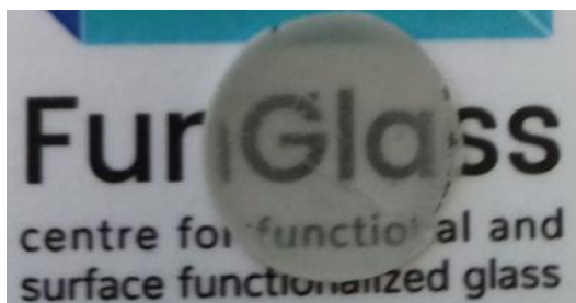
Fig. 1 Bulk glass in the composition of YAG + 24 wt. % \text{Al}_2\text{O}_3 sample sintered in viscous flow.
